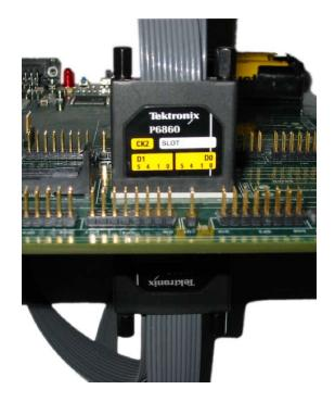
PCB with back-to-back P6860 probes installed
